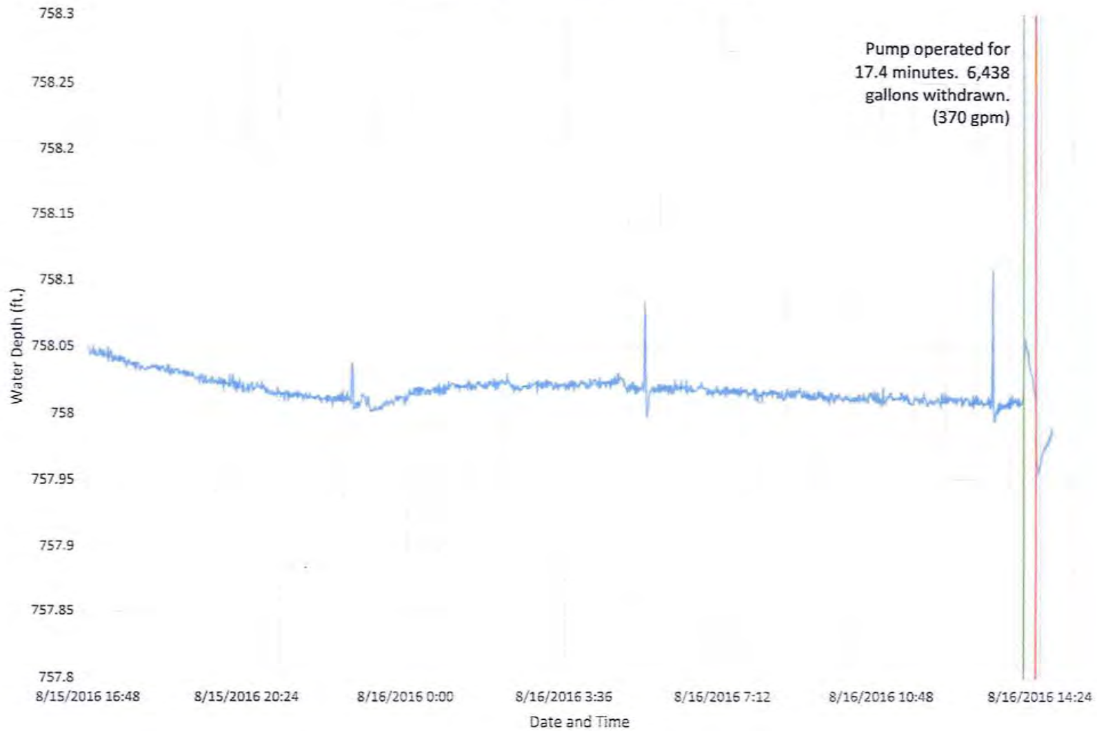
Figure 15 Water Level Data Recorded - MW-30D
